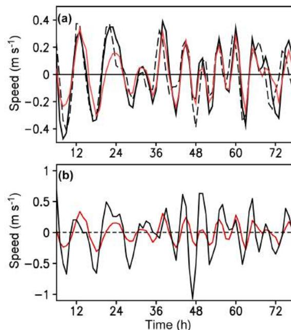
**Figure 14.** Fluctuations (deviation from the 9 h running mean) of (a) the tropical cyclone speed (black solid), the PVT speed (black dashed) and the difference between the tropical cyclone speed and the conventional steering (red solid), and (b) the difference between the tropical cyclone speed and the conventional steering (red solid), and the difference between the contribution of the HA term and the conventional steering (black).
