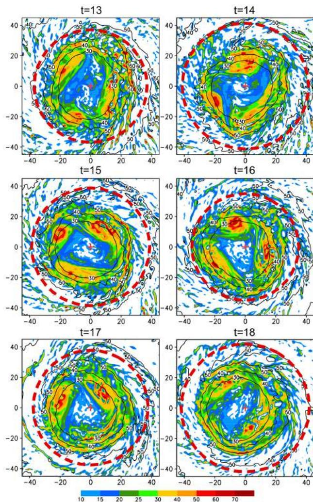
**Figure 13.** Distribution of potential vorticity (shaded,  $10^{-6} \text{ m}^2 \text{ s}^{-1} \text{ K kg}^{-1}$ ) and magnitude of wind (contour,  $\text{m s}^{-1}$ ) within the inner-core region during the period of 13–18 h at 700 hPa. The dashed circle shows the radius of maximum wind, with the tropical cyclone center indicating with crosses.
