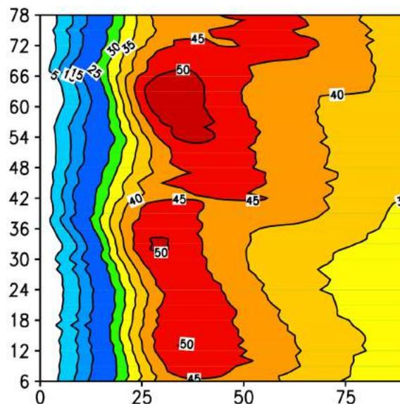
**Figure 4.** Evolution of the simulated azimuthal mean component ( $\text{m s}^{-1}$ ) of the 700 hPa wind in the 9 km domain. The  $x$  axis and  $y$  axis indicate the distance (km) from the storm center and the integration time (hours), respectively.
