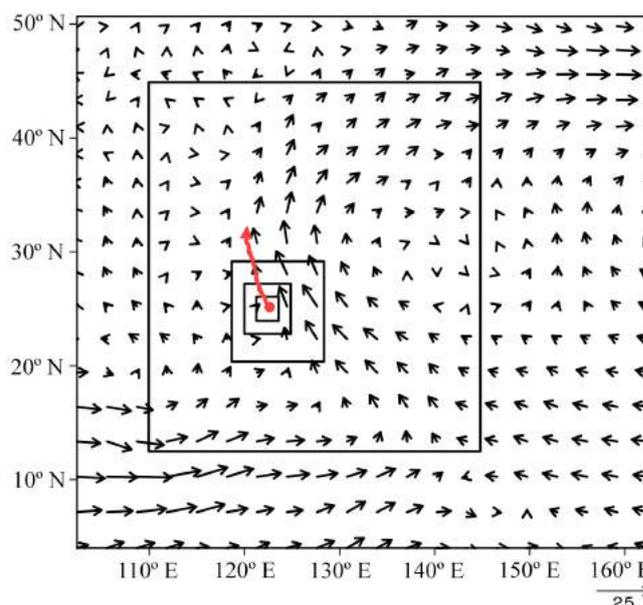
**Figure 1.** Model domains of the numerical experiment with the three innermost domains moving with the storm, the initial 850 hPa wind ( $\text{m s}^{-1}$ ) field (vectors) and the simulated tropical cyclone track (red).
