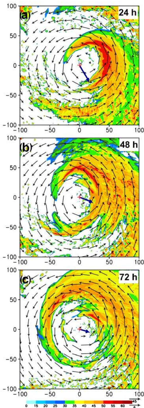
**Figure 3.** Simulated wind (vectors,  $\text{m s}^{-1}$ ), radar reflectivity (shading, dBz) fields at 700 hPa, and the vertical wind shear (bold arrows in the center) between 200 and 850 hPa after (a) 24, (b) 48 and (c) 72 h integration. The  $x$  and  $y$  axes indicate the distance (km) relative to the storm center. The upper (lower) scale vector at the right lower corner is for the 700 hPa wind (vertical wind shear).
